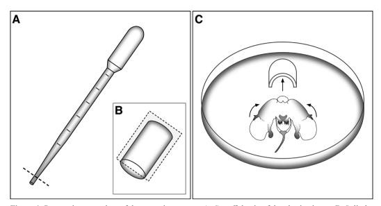
Figure 1. Preparation procedure of the mounting system. A. Cut off the tip of the plastic pipette; B. Split the small piece of pipette into two halves; C. Attach one of the halves on the bottom of the petri dish and fix the genitalia in the generated tunnel. Dashed lines indicate the cuts.
